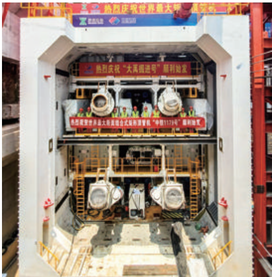
中国中铁研发的世界最大断面组合式矩形顶管机“大禹掘进号”始发 The world's largest cross-section combined rectangular pipe jacking machine "Dayu Tunneling" developed by CREC was put into use
